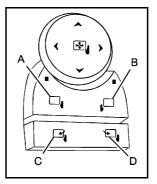
Vehicles with outside power mirrors and foldaway mirrors have controls located on the driver door.
